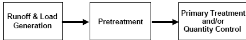
FIGURE 4-34 Generalized Stormwater Treatment Train
